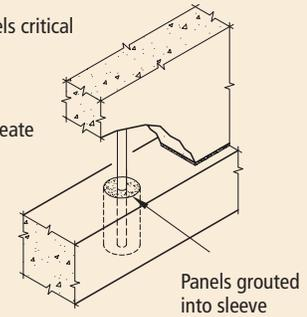
Fig. 4.5.73 Bearing wall to foundation (BWF4).
