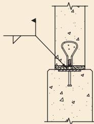
Fig. 4.5.72 Bearing wall to foundation (BWF3).
