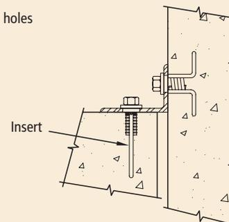
Fig. 4.5.41 Bolted tieback (BTB5).
