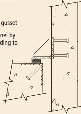
Fig. 4.5.26 Eccentric bearing (EB4).
