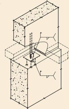
Fig. 4.5.74 Bearing wall to foundation (BWF5).
