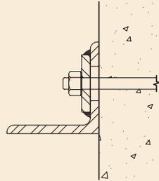
(b) Loose plate under angle, welded after adjustment eliminates bending in bolt
