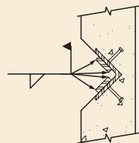
Fig. 4.5.52 Panel to panel alignment (PPA1).
