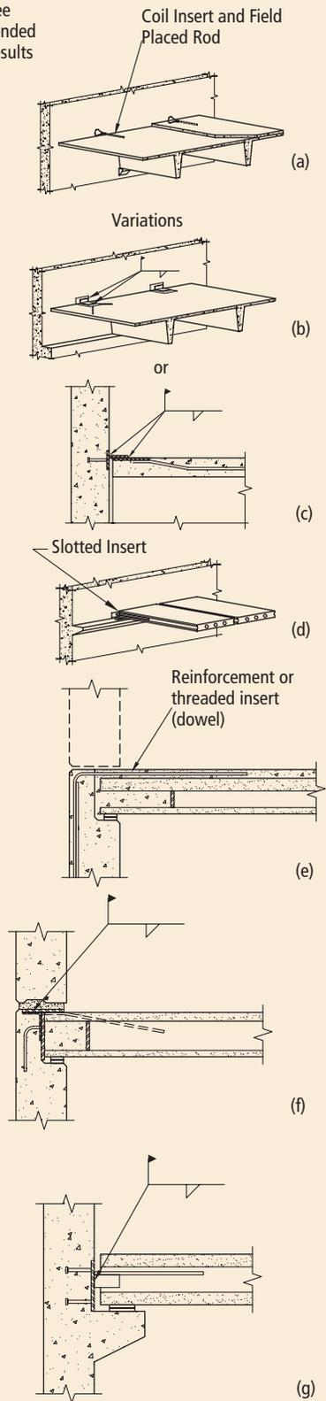
Fig. 4.5.76 Slab to bearing wall (SBW2).
