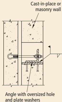
Fig. 4.5.45 Shear plate (SP1).
