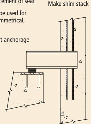
Fig. 4.5.24 Eccentric bearing (EB2).
