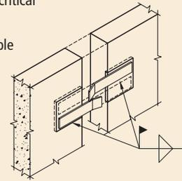
Fig. 4.5.53 Panel to panel alignment (PPA2).
