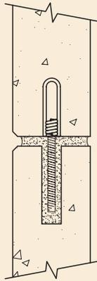
Fig. 4.5.20 Direct bearing (DB6).
