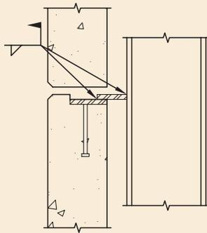
Fig. 4.5.33 Welded tieback (WTB5).
