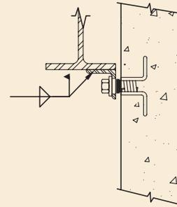
Fig. 4.5.37 Bolted tieback (BTB1).
