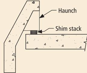
Fig. 4.5.18 Direct bearing (DB4).
