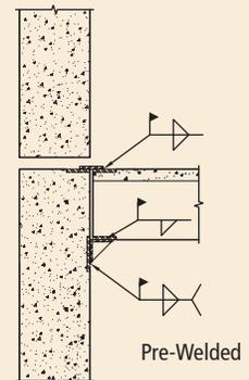
Fig. 4.5.78 Slab to side wall (SSW1).
