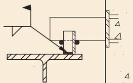
(c) Use in pairs. Round bar shop welded to bearing bracket.
