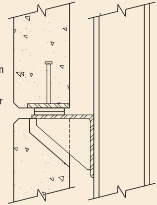
Fig. 4.5.19 Direct bearing (DB5).
