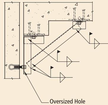
Fig. 4.5.31 Welded tieback (WTB3).
