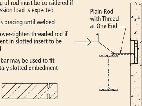
Fig. 4.5.34 Welded tieback (WTB6).
