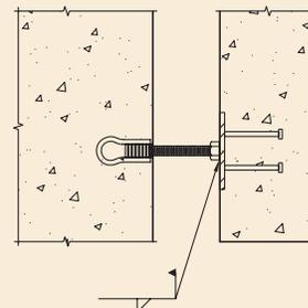
Fig. 4.5.35 Welded tieback (WTB7).
