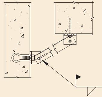
Fig. 4.5.30 Welded tieback (WTB2).
